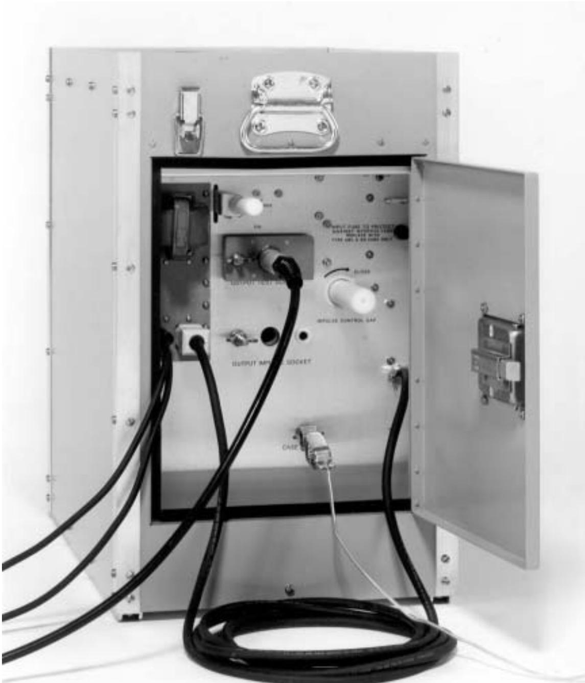
Photograph of the unit set up for cable testing and operation from its inverter. The combination high voltage output and ground return cable goes off to the left. A ground must be connected to the case. The input power cord is plugged directly into the inverter. The battery leads go to a 12 volt battery with red to positive and black to negative.
