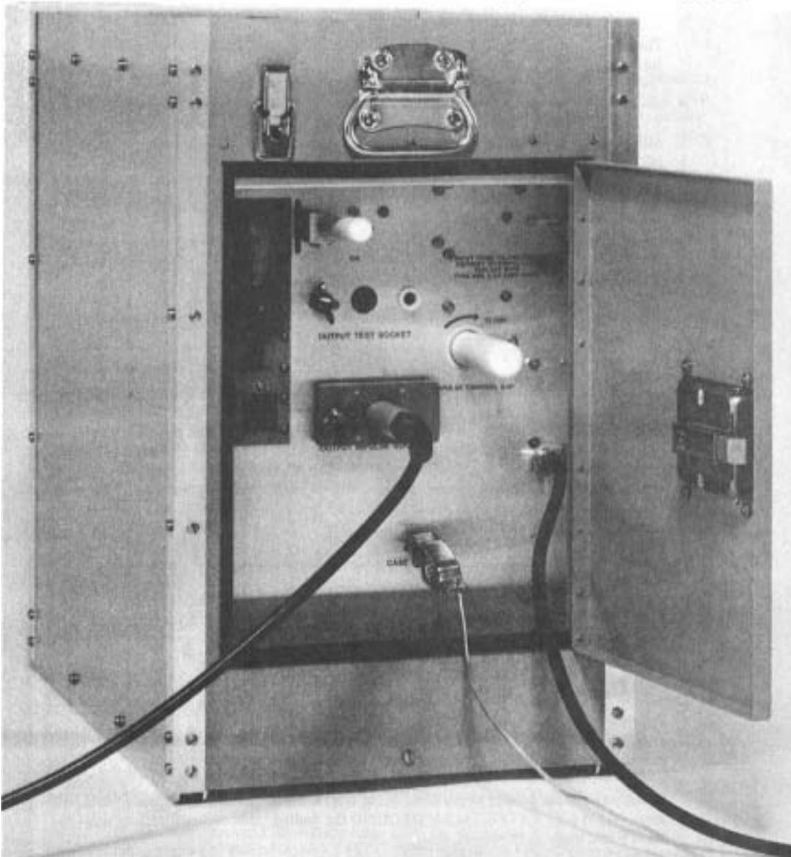
Photograph of the unit set up for cable fault locating. The high voltage output and ground return cable goes off to the left. The input power cord is off to the right. The required ground lead to the case goes off to the right. The main ground return through the test lead should be connected solidly to the neutral of the cable to be thumped and the system neutral. The impulse control gap handle is located in the right corner of the lead compartment to the right of the output impulse socket.
